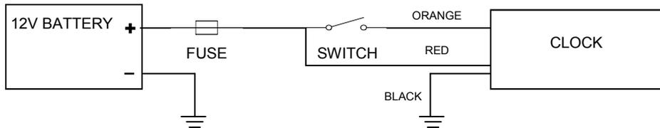
As usual best practise, please ensure all + wiring is fused as near as possible to the voltage source and run in a workmanlike manner. All connections must be secure, low resistance and protected.
