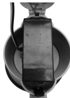
Rechargeable battery position
